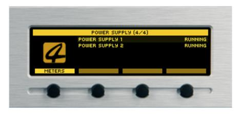
Section Power Supply - contains information as regards the Power Supply 1 & 2 state.
